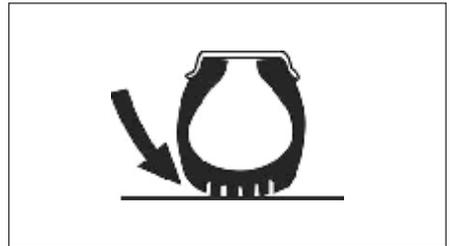
**Important:** According to tire manufacturers' specifications, tire pressure must be calibrated when tires are COLD (allow the tires to cool for 3-4 hours after use). Tire pressure may increase up to 12 % over the "cold" pressure due to rolling resistance when in use. VIGIA will show this pressure increase in the control panel's gauges. DO NOT BLEED THE TIRES.
