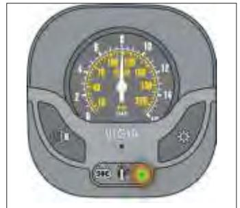
**Yellow L.E.D. (flashing):** Tire punctured or air leak. The system is recuperating the air loss and driver can continue the trip.
