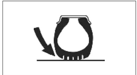
**Important:** According to tire manufacturers' specifications, tire pressure must be calibrated when tires are COLD (allow the tires to cool for 3-4 hours after use). Tire pressure may increase up to 12 % over the "cold" pressure due to rolling resistance when in use. VIGIA will show this pressure increase in the display module's gauges. DO NOT BLEED THE TIRES.
