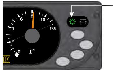
**Yellow L.E.D. (flashing):** Tire punctured or air leak. The system is recuperating the air loss and driver can continue the trip.
